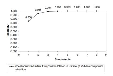
**Fig. 1.** The benefits of redundancy for reliability.
